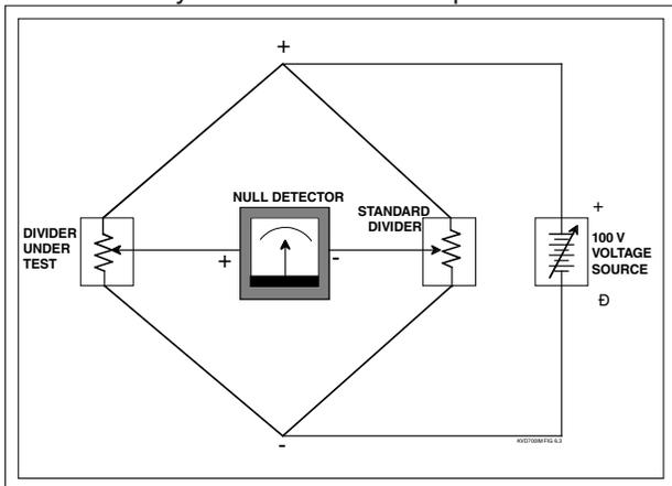
Typical application of a Kelvin-Varley Voltage Divider for measuring resistance of voltage
