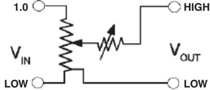
Linearity deviation, the error between the actual output voltage ( $V_{OUT}$ ) and the output voltage for a particular setting ( $S$ ) =  $[V_{OUT}/V_{IN}] - S$ . Linearity will be smaller than the resistor accuracy.
