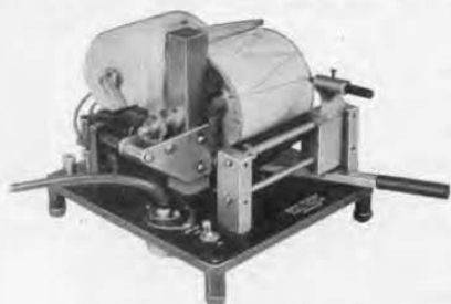
TYPE 459-A Manual Recorder. Moving the handle simultaneously moves the pen and the slider on a potentiometer
