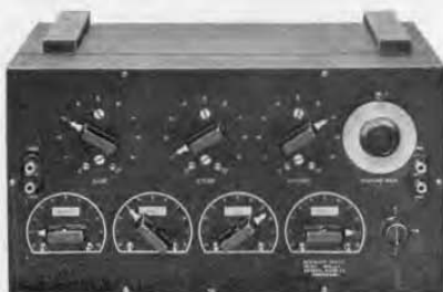
FIGURE 1. An adjustable resonant circuit, a typical application of TYPE 510 Decade-Resistance Units and TYPE 380 Decade Switches and Condensers
