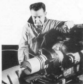
This is how General Radio winds copper tubing in the manufacture of a TYPE 679-A Inductor
