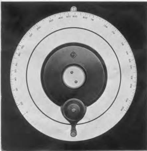
FIGURE 1. This dial is used with TYPE 739-A Logarithmic Condenser in the TYPE 713-B Beat-Frequency Oscillator. The scale is logarithmic between 20 and 20,000 cycles.
