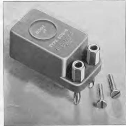
FIGURE 2. TYPE 505 Condenser has plug-in terminals as shown here. In a measuring circuit equipped with jacks, condensers can be easily changed, or stacked in parallel. The voltmeter probe plugs into the jack tops of the condenser terminals.
