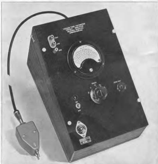
FIGURE 1. Panel view of the TYPE 726-A Vacuum-Tube Voltmeter, showing the probe in which the diode is housed.
