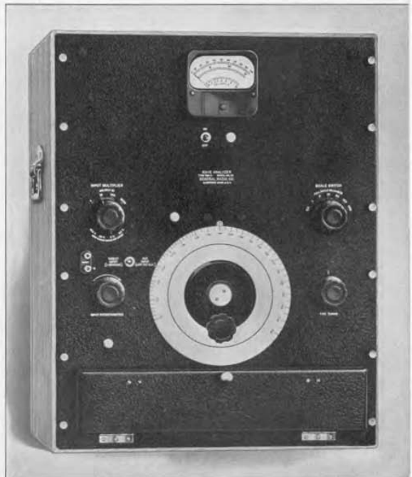
FIGURE 1. Panel view of the TYPE 736-A Wave Analyzer. The panel is standard 19-inch relay-rack width.
