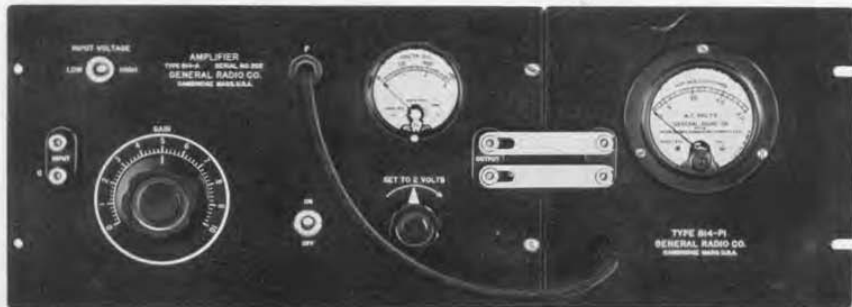
FIGURE 1. The TYPE 814-AR Amplifier with meter and filter. The filter can be mounted at the rear of the instrument, and is connected to the panel jack through a hole in the panel
