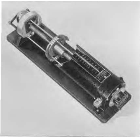
FIGURE 2. Cut-away view of TYPE 757-A Ultra-High-Frequency Oscillator, showing the internal construction.
