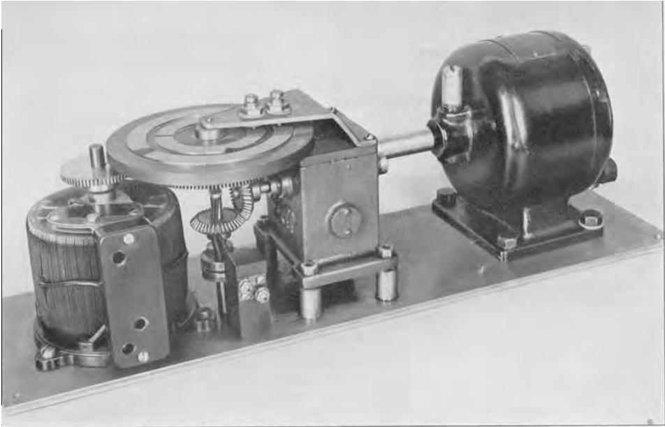
View of a motor-driven Variac with automatic limit attachment.
