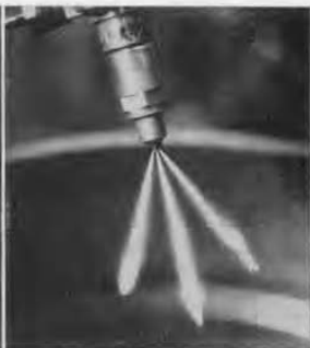
Figure 14. Strobotac single-flash photo of the fuel-injection spray of Figure 11. The bright, easily triggered flash makes it easy to take permanent records of observed phenomena.
