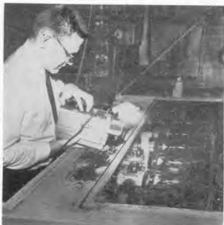
Figure 9. The bright Strobotac beam penetrates both an oil bath and the tube envelope to illuminate a rotating-anode X-ray tube at Machlett Laboratories.
