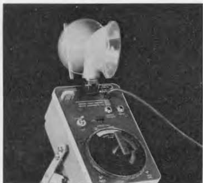
Figure 5. This multiple-exposure photograph illustrates the 360-degree reflector rotation. Hinged lamp assembly permits additional positioning in vertical plane.
