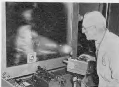
Figure 8. The Strobotac produces enough light to "stop" the motion of the fan through the eight layers of glass in the door of this altitude chamber. Some reflection is produced by the glass layers, but its effect is minimized by aiming the Strobotac flash into the chamber at an angle rather than head on. The new instrument's increased speed range now makes it possible to measure directly the speeds of fans operating at 400 cycles (24,000 rpm), which are commonly used in aircraft.
