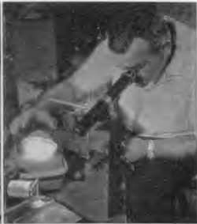
Figure 12. At General Electric's Small Aircraft Engine Department, engineers use the Strobotac to examine the vibratory modes in aircraft gas turbine blades. The short-duration white light gives excellent resolution. Mode shapes are clearly defined at various excitation frequencies produced by an electromagnetic driver.
