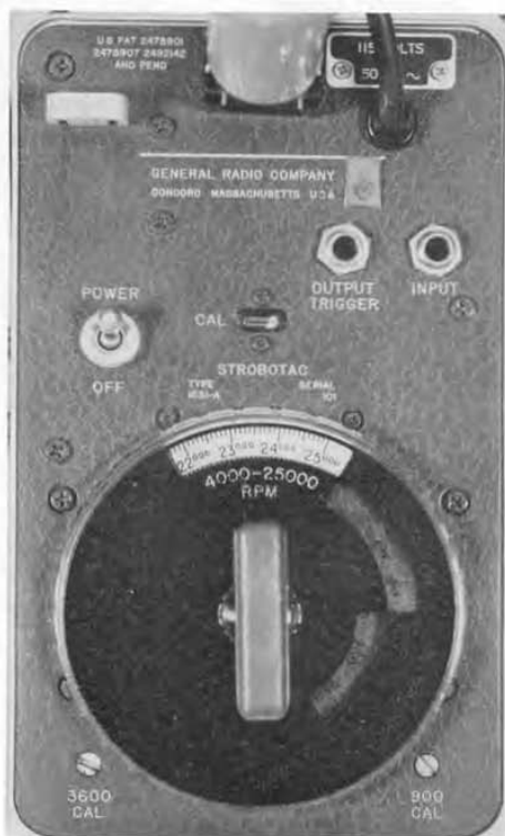
Figure 6. View of the panel, showing scale, mask, dial, and other conveniently arranged controls.
