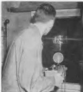
Figure 13. A model helicopter rotor in a wind tunnel is watched with the Strobotac. Blade lag and flapping are clearly observed in slow motion, just as they occur under various flight conditions. In addition to providing a good visual representation of the conditions encountered in flight, such studies serve as a visual check on vibration data provided by strain-gages mounted on the rotor head.
