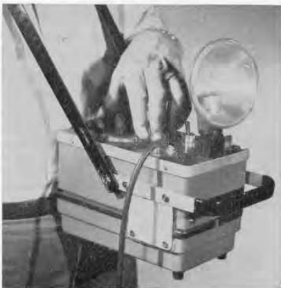
Figure 4. This adjustable neck strap supplied with the Strobotac frees the operator's hands for other functions.
