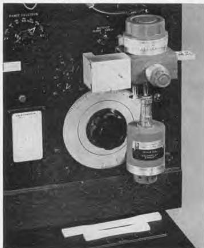
Figure 1. Standard tensile bar in dielectric sample holder. Pin in jig acts as stop for shorter specimen.
