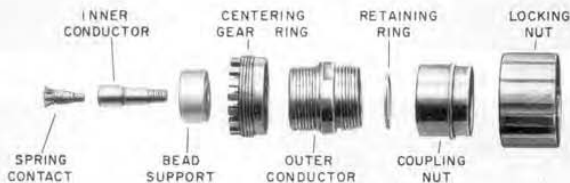
Figure 1. Exploded view of the Type 900-BT Precision Coaxial Connector.
