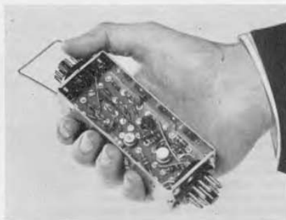
Figure 1. Multipurpose plug-in code modules with individual input connectors allow complete freedom for composing a desired printing format.
