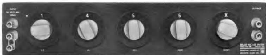
Figure 1. Type 1455-BH Decade Voltage Divider.
