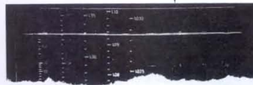
Figure 5. Typical calibration curve for insertion-loss measurements in 2.0- to 4.0-GHz range; full scale = 0 dB.
