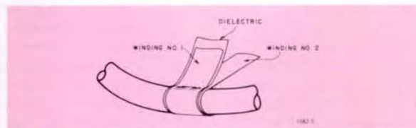
Figure 4. Flat-conductor transformer-winding design.
