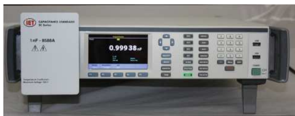
Figure 3-7: SCA -8588A on the Fluke 8588A
